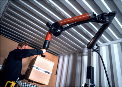
Low-built articulated arm in either steel or carbon with a height reach of 2.1m to 2.6m
