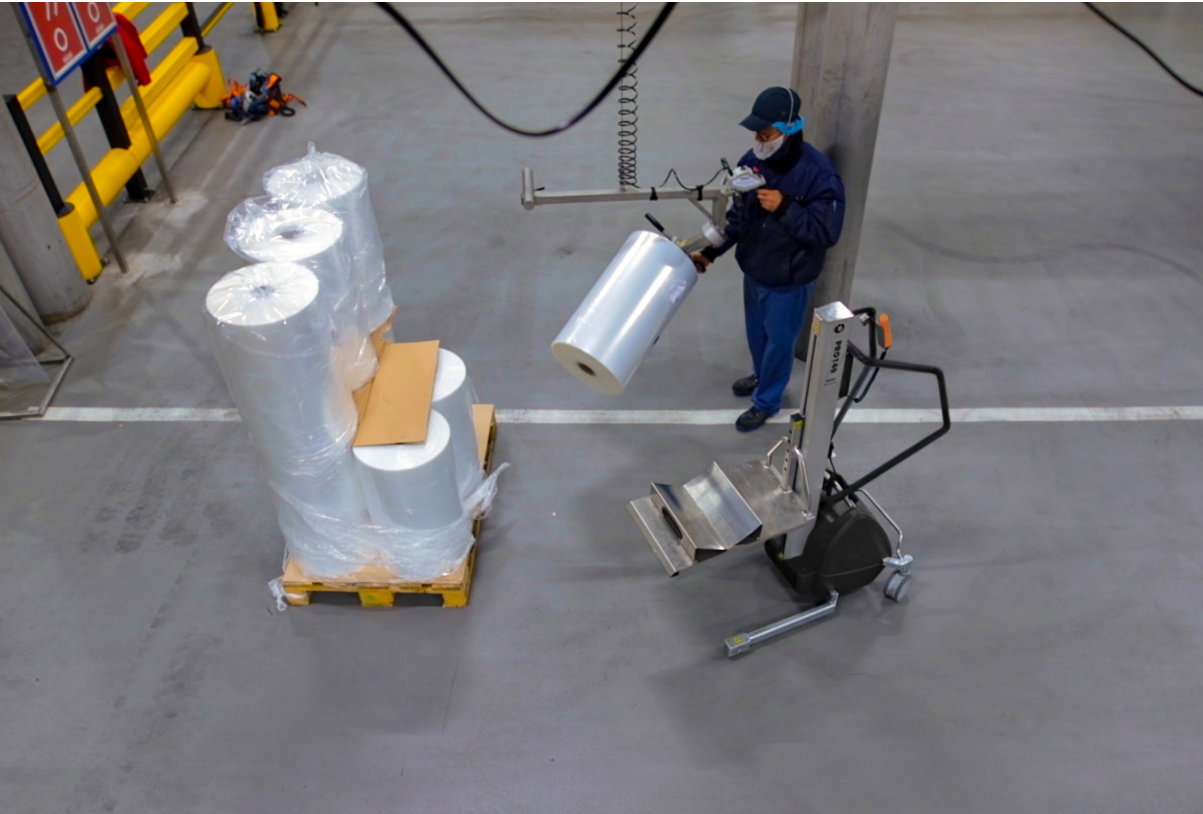
The hoists can be easily combined with other TAWI lifting solutions. Here the wire hoist is used to lift heavy film rolls from a pallet, tilt them and then put them on a portable trolley. The trolley is then used for transporting and mounting the rolls into packaging machines.
