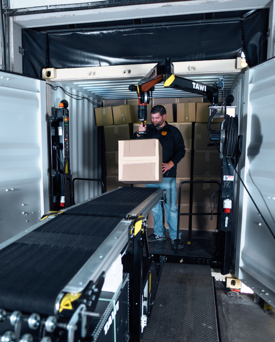
The container unloader+Loader has a stabilised system with built-in balancing to help when traveling over inclines.
