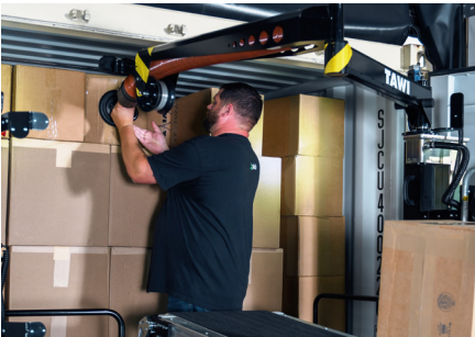
The adjustable platform makes it easily to reach all boxes in the container, from top to bottom.
